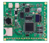
The GDB-03 training kit allows you to learn both the basic and the advanced functions of the GDS-3000 Series Digital Storage Oscilloscope (DSO). Following the training procedures of this training kit, you will quickly understand the basic operations of a DSO, and the unique features of the GDS-3000 Series, which represents a typical hi-tech DSO today.
