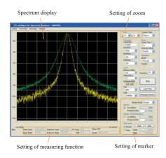
MAS400 is a software that controls the spectrum analyzers of four models by the PC. 1001 points are captured in the spectrum analyzer. Although 501 points are displayed on its screen, the number of points transferred to the PC is all of 1001 points.
