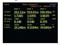
When the INTEG mode is selected, true and fundamental values of all integrated values are presented. Using the NEXT and BACK buttons, any individual phase or the sum value of all phases can be viewed.
