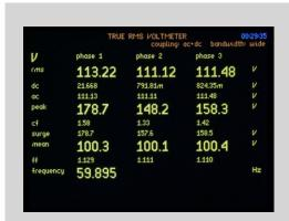
In addition to the true rms value of voltage and current on any measurement channel, RMS mode also provides real time analysis of dc, ac, peak, crest factor, surge, mean and form factor.
