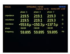
Utilising true real time DFT analysis, the PPA5500 provides precision impedance measurements on any individual phase or a simultaneous display of all three phases as shown here.
