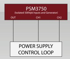
As illustrated above, the PSM3750 eliminates the requirement for an isolation transformer and differential probes. Another disadvantage when performing analysis over a wide frequency band is that many different isolation transformers will be required for the different frequency ranges of the test, the PSM3750 eliminates this problem and generates frequencies throughout its entire frequency range from a single output.
